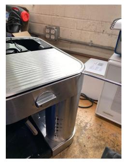
Once you have the top lid off, you will be able to access the steam valve, pump and boiler of the unit to service.
