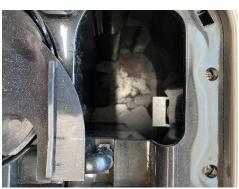
Remove the screws from around where the water is poured in on the drip side. Note there is a hidden screw behind the hinged lid part. You need to pull back on the shower cap and remove from the lid to be able to access this screw and remove. Remove all the screws around the top.
