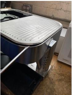
Take a flat screwdriver and wedge between the top part and pull up. Note the top lid has clips that press it in so you need to pop up and pull. Do on both sides of the unit and then you should be able to remove the top lid.
