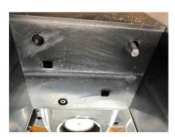
Now you need to remove the 2 screws by where the water tank goes.
