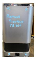
2) After those screws are removed, you will have to pull the 3-sided housing back away from the unit as it is snapped to the front. Then pull the housing from the back away from the unit.
