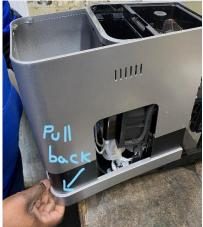
3) Then you will have to unlatch the 3 sides with a flat screwdriver. Follow below steps and then lift the top chrome housing.
