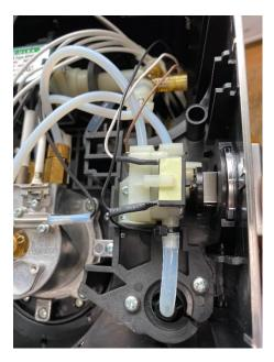
Once you have remove the top housing, you will be able to see the steam valve assembly of the EM Series.
