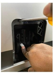
With the unit OFF, you will need to place a screwdriver or even can use folded piece of cardboard to press in microswitch. Then you will need to press in the button on the round white gear.
